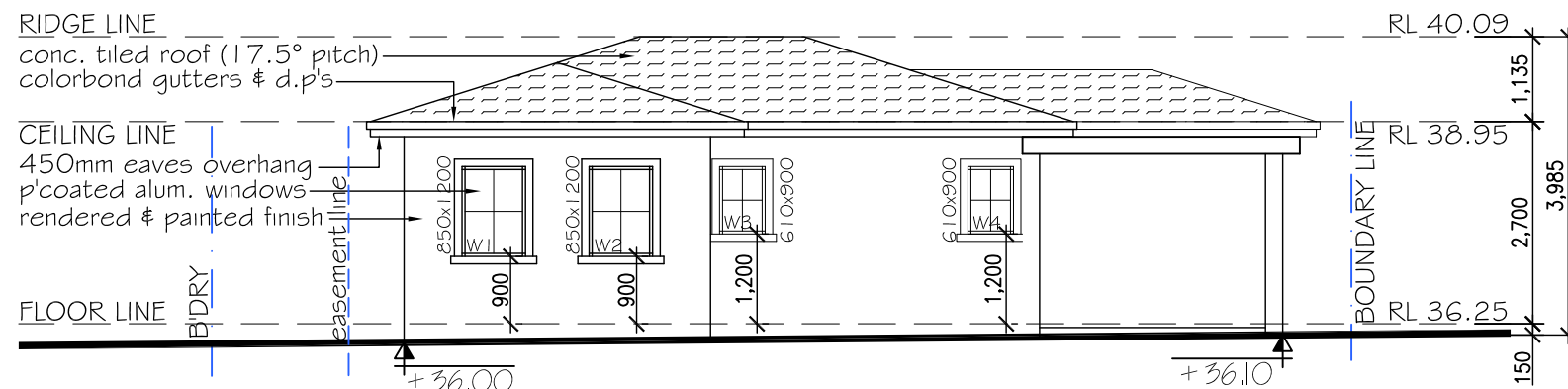
EAST ELEVATION (secondary dwelling) SCALE 1: 100
